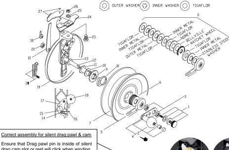
drag cam slot or reel will click when winding. Spring loop to go over pin for correct operation of the drag.
